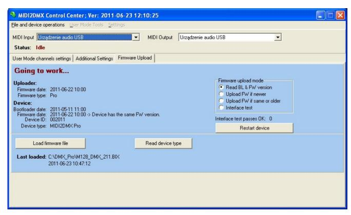
In general most operations on this tab are active during power-up of the device, however in the User Mode [Mode 8] user can restart device using **Restart device** button.
