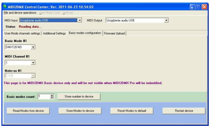
The above screen shows **Basic modes configuration** tab after the application start before the current set up is read from the device.
