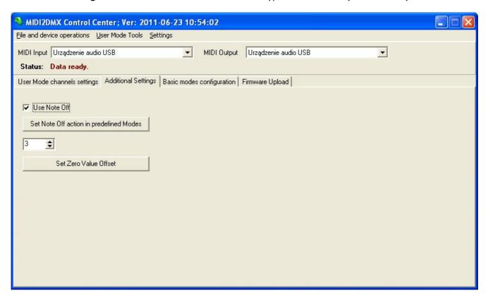
**Use Note Off -** DMX channel value is set using Note On Velocity or Control Change value. The user may also activate Note Off function which works like Note On with velocity equals 0 (zero). This setting is active for predefined modes (0-7) and for User Mode **[8 - DMX512 UM]**.
