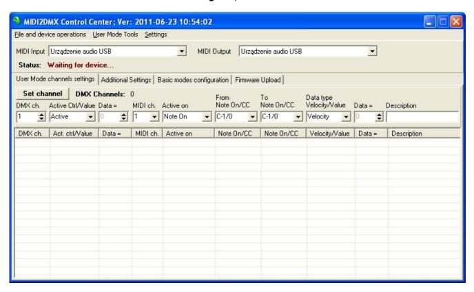
Preparing device to work with MIDI2DMX Control Center expect two MIDI connections between device and MIDI interface in "closed loop" fashion. It means that MIDI IN from device should be connected to MIDI OUT of the computer's MIDI interface and device's MIDI OUT should be connected to MIDI IN connector of the computer's interface.
